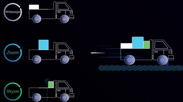
Wi-Fi 6 uses OFDMA, an extension of the OFDM architecture, to improve data-rate efficiency and reduce latency for densely-connected wireless networks, such as IoT environments for Smart industrial applications. OFDMA can significantly boost data throughput and reduce wireless latency by achieving highly-efficient spectral usage across the wireless signal.
