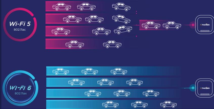
MU-MIMO, to further reduce network latency and significantly increase wireless network bandwidth. Earlier versions of Wi-Fi 5 used SU-MIMO\* (Single User Multiple Input Multiple Output), which only allowed communication with multiple devices in consecutive order, or one at a time. Wi-Fi 6 with MU-MIMO uses multiple spatial streams for simultaneous communication with multiple devices which greatly improve both upload and download performance.
