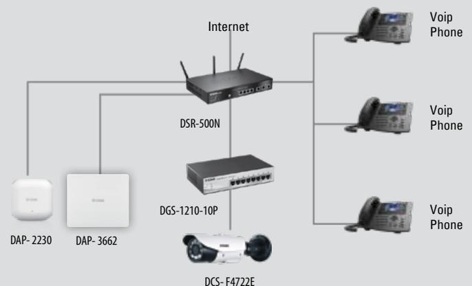
PoE devices can transmit a Discovery Protocol that informs the PoE Switch of the actual power required by the device. If the power is less than the default (15.4W for PoE or 30 W for PoE+), the PoE switch acknowledges the request with its available power and modifies the power budget accordingly. If the requesting powered device exceeds the power budget for the switch, the port is either powered down, or the port remains in low-power mode.
